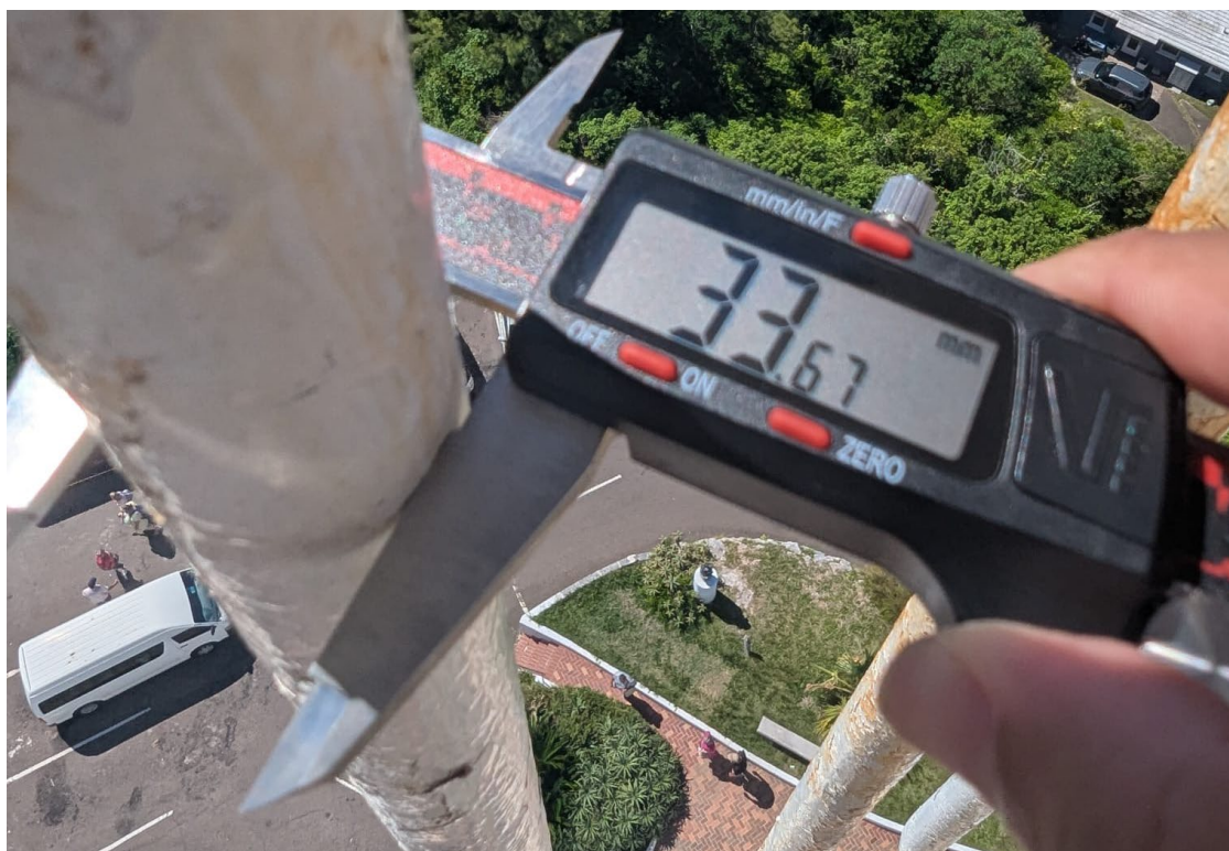
Photograph 26: Bar 130 diameter (mid-point of bar - measured in millimetres)
